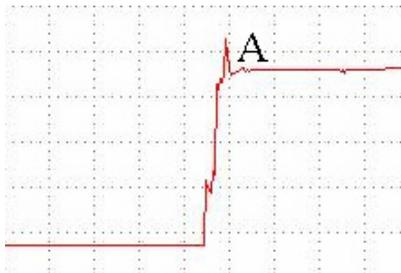
Capturing current flow measurements in this manner shows how the parasitic draw changes over a period of time. The flat line on the left side is zero amps. No current is flowing. The rise in the center is current flow starting as the battery cable was connected. Point A shows that after the battery cable was reconnected the vehicle’s control modules were drawing approximately two amps. From left to right, start to finish, a nine second period of time is shown.
